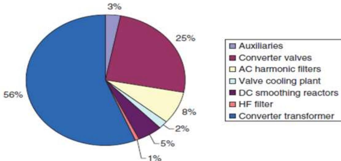
Figure: 2 break down LCC converter Station loss
