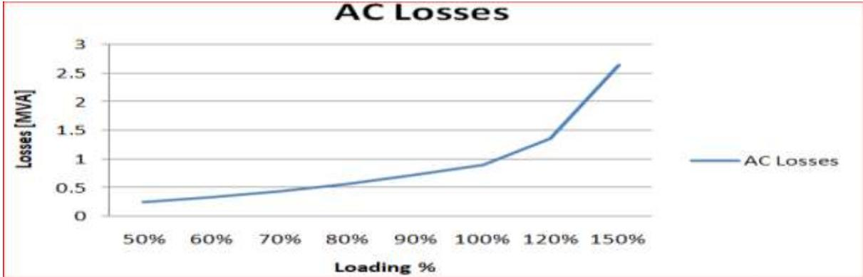
Figure 8: AC System Losses under different loading conditions
